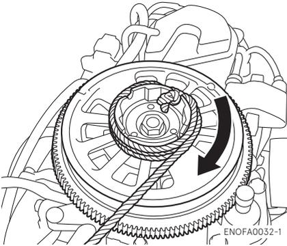
5. Tie a loop in the another end of the emergency starter rope and attach socket wrench, Both the loop and the wrench are provided in outboard motor box.
