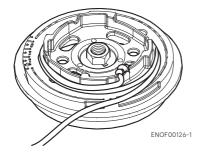
Tie a loop in the another end of the emergency starter rope and attach socket wrench that is included in the tool kit.
