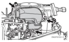
Remove starter lock cable from recoil starter by pulling the starter lock cable.
