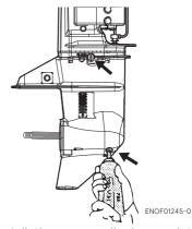
4. Install the upper oil plug, and then remove oil tube nozzle and install the lower oil plug.
