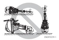
Keep the outboard motor in a vertical position when carrying.
