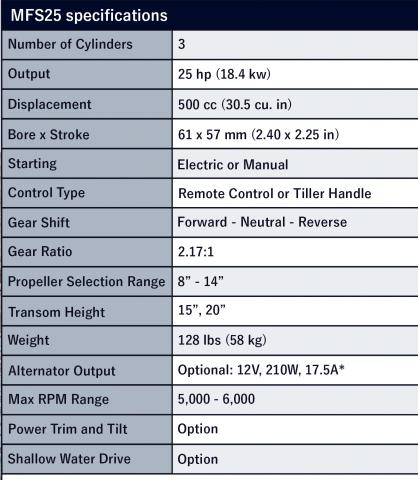
Standard features include: Electronic Fuel Injection, Digital CD Ignition System, Start in Gear Protection, Thermostat Controlled Cooling System, Through-The-Prop Exhaust, Oil Pressure Warning, and Variable Idle Speed
