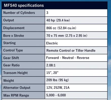
Standard features include: MicroComputer Programmed Ignition System, Electronic Fuel Injection, Start in Gear Protection, Thermostat Controlled Cooling System, Through-The-Prop Exhaust, Overheat Buzzer, Power Trim and Tilt, Oil Pressure Warning, and Variable Idle Speed.
