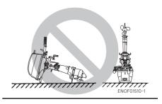
Keep the outboard motor in a vertical position when carrying.
