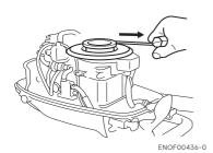
9. After engine starts, do not reinstall recoil starter and top cowl.
